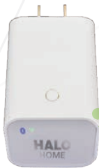
internet access bridge
