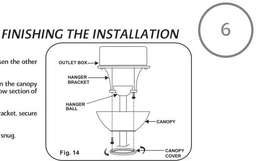
Step 1. Remove 1 of the 2 screws from the bottom of the hanger bracket and loosen the other one half a turn from the screw head.
